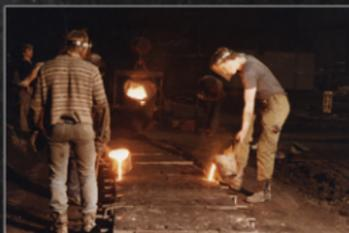
Moulders pouring metal into moulding boxes with hand ladles, 1984
