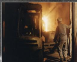
Filling container with molten metal at cupola spout, 1984. A Hyster truck is supporting the container while it is filled with molten iron.
