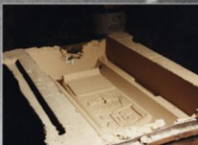
Moulding box with mould for pillar box, 1984
