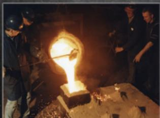
Molten iron being poured from ladle into moulding box, 1984
